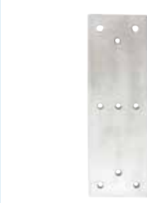
Back plate. Galvanized 750 x 250 x 15 mm Weight: 24 kg
