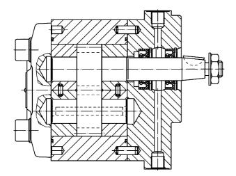
Depending on the medium to be transferred, operating pressures up to 150 bar are possible with driving speeds of about 1500 rpm.
