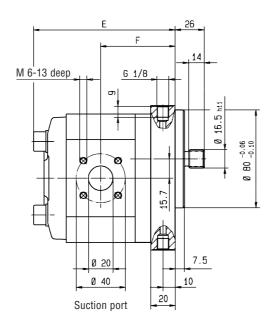
Shaft end: Involute spline B 17 x 14 DIN 5482 but tooth thickness  $s_w = 3.206$  Addendum modification = +0.6
