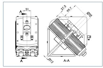
The CB-Version with central clearance hole provides the relocation of wires through the swivel head by the customer. Please note, that improper wire-relocation frequently leads to wire-damages. The inset of the swivel head with integrated transmission leadthrough "EDF" is long-lasting and safe .
