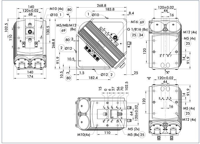
The main view shows the SRH in the version with integrated transmission leadthrough EDF. The swivel head is drawn in the left end position (0°) and turns clockwise till 180°. (view on the output side)
