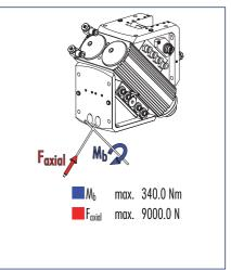
① Moments and forces may occur simultaneously. When using heavy attachments or ones with high mass moments of inertia, the speed must be restricted to ensure that the rotary movement occurs without any hitting or bouncing.
