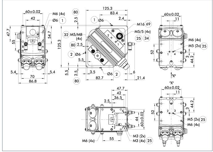
The main view shows the SRH in the version with integrated transmission leadthrough EDF. The swivel head is drawn in the left end position ( $0^\circ$ ) and turns clockwise till 180°. (view on the output side)
