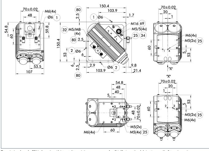
The main view shows the SRH in the version with integrated transmission leadthrough EDF. The swivel head is drawn in the left end position (0°) and turns clockwise till  $180^{\circ}$ . (view on the output side)
