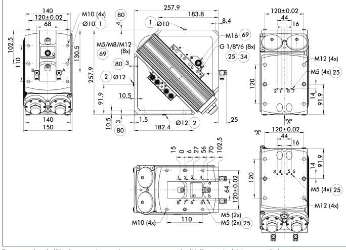
The main view shows the SRH in the version with integrated transmission leadthrough EDF. The swivel head is drawn in the left end position (0°) and turns clockwise till  $180^{\circ}$ . (view on the output side)
