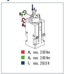
① The indicated moments and forces are static values, apply per base jaw and may occur simultaneously. My may arise in addition to the moment generated by the gripping force itself. If the max. permitted finger weight is exceeded, it is imperative to throttle the air pressure so that the jaw movement occurs without any hitting or bouncing. Service life may be reduced.
