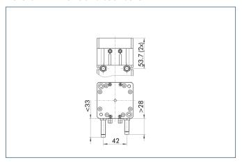
The drawing shows changes in dimensions of the shock absorber versions, compared to the elastomer versions shown on the main view.
