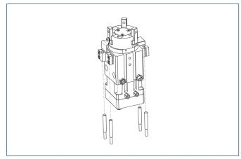
End position monitoring mounted with mounting kit
