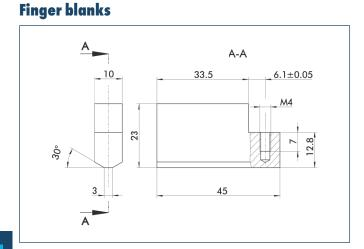
Finger blanks for customized subsequent machining
