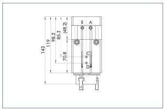
The mechanical gripping force maintenance device ensures a minimum gripping force even in case of pressure drop. This acts as closing force in the AS version, and as opening force in the IS version. In addition, the gripping force maintenance device can also be used for increasing the gripping force or for single-acting gripping.
