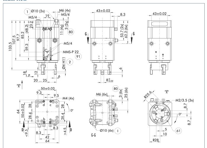
The drawing shows the gripper in the basic version with opened jaws without considering the dimensions of the described options below.
