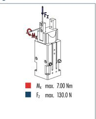
The indicated moments and forces are statical values, apply for each base jaw and should not appear simultaneously. If the maximum admissible finger weight is exceeded, throttling is necessary in order to ensure a smooth jaw motion without jerks or bounces. The life-time may reduce.
