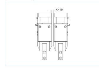
CAUTION: Monitoring is carried out by magnetic switches, and in case of side-by-side assembly of several units, a minimum distance of X mm between the units must be maintained.
