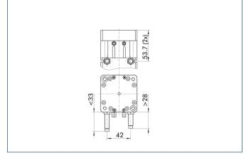
The drawing shows changes in dimensions of the shock absorber versions, compared to the elastomer versions shown on the main view.
