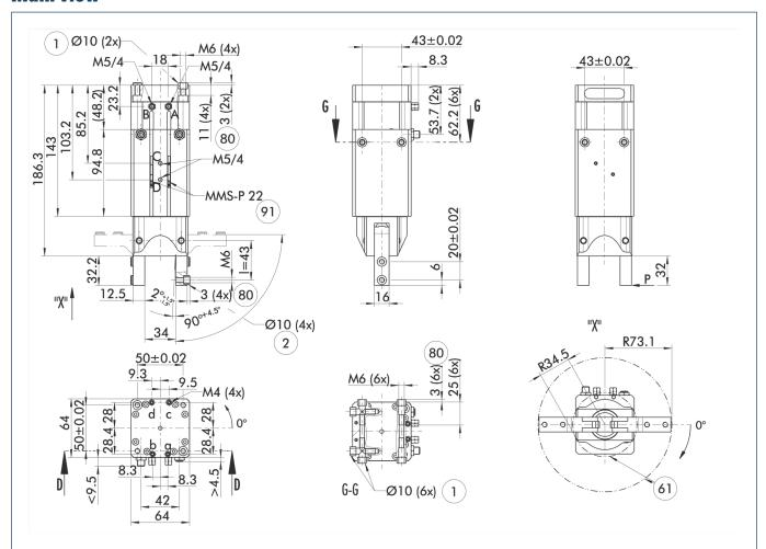
The drawing shows the gripper in the basic version with closed jaws, the dimensions do not include the options described below.
