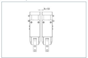
CAUTION: Monitoring is carried out by magnetic switches, and in case of side-by-side assembly of several units, a minimum distance of X mm between the units must be maintained.
