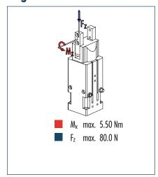
The indicated moments and forces are statical values, apply for each base jaw and should not appear simultaneously. If the maximum admissible finger weight is exceeded, throttling is necessary in order to ensure a smooth jaw motion without jerks or bounces. The life-time may reduce.
