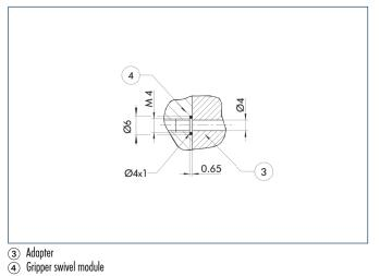
The direct connection is used for supplying compressed air without hoses. Instead, the pressure medium is fed through bore-holes in the mounting plate.
