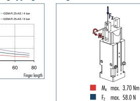
The indicated moments and forces are statical values, apply for each base jaw and should not appear simultaneously. If the maximum admissible finger weight is exceeded, throttling is necessary in order to ensure a smooth jaw motion without jerks or bounces. The life-time may reduce.
