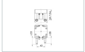
The drawing shows changes in dimensions of the shock absorber versions, compared to the elastomer versions shown on the main view.
