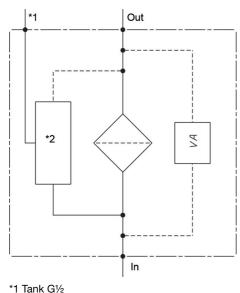
\*2 Cold start valve VA = Maintenance indicator In = G1 Out =G1 We recommend to contact us concerning applications of our filters in areas governed by the Eu Directive 94/9 EC (ATEX). The standard version can be used for liquids based on mineral oil (corresponding to the fluids in Group 2 of Directive 97/23 EC Article 9). If you consider to use other fluids please contact us for additional support.
