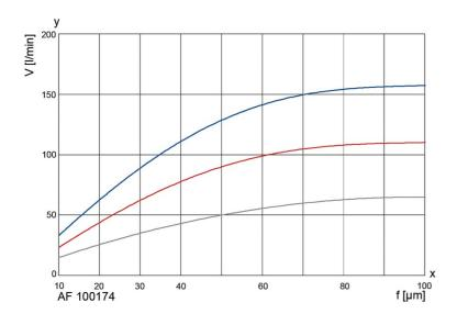
The curves indicate the volume flow through the complete filter system (filter housingh including element) and are referred to a differential pressure of 0.3 bar. Specific process information is essential to guarantee reliable operation of an automatic filter.
