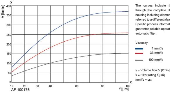
The curves indicate the vclume flow through the complete filter system (filter housing including element) and are referred to a differential pressure of 0.3 bar. Specific process information is essential to guarantee reliable operation of an
