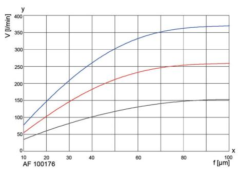
The curves indicate the volume flow through the complete filter system (filter housing including element) and are referred to a differential pressure of 0.3 bar. Specific process information is essential to guarantee reliable operation of an automatic filter.
