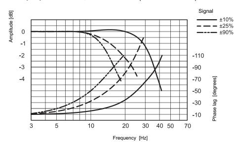
These test amplitude are performed with 50% of max flow, and  $\Delta p$  (P-T) 10 bar.
