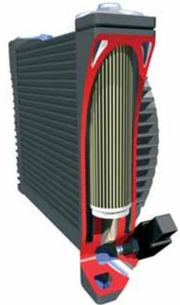
*By integrating a bypass system in an asa radiator, it is possible to avoid overstressing the cooler at coldstart conditions (due to extremely viscous oil). This mode of construction also allows high oil flows through the cooler, which for example can occur when using differentiated hydraulic cylinders.*
